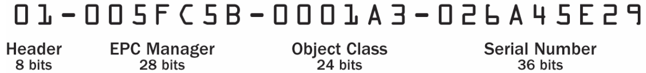
Figure 5-1. Example 96-bit EPC
